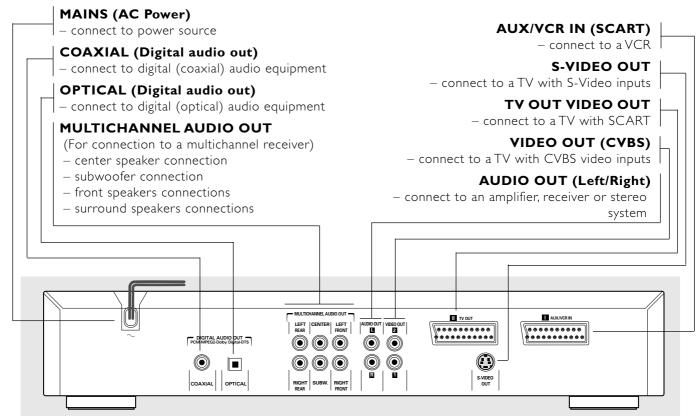
Caution: Do not touch the inner pins of the jacks on the rear panel connectors. Electrostatic discharge may cause permanent damage to the unit.
